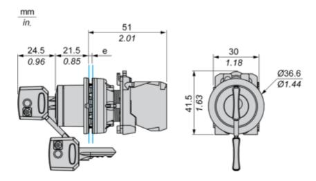
$\boldsymbol{e}\text{:}$  Clamping thickness: 1 to 6 mm / 0.04 to 0.24 in.
