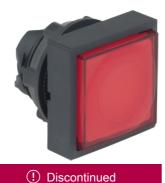
Head for illuminated push button, Harmony XB5, red square projecting illum pushbutton Ø22 mm spring return integral LED
