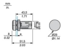
e Support panel thickness: 1 to 6 mm/0.4 to 0.24 in. (metal), 2 to 6 mm/0.8 to 0.24 in. (plastic).
