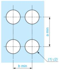
(1) Diameter on finished panel or support (2) Ø22.5 mm recommended (Ø22.3  $_0^{+0.4}$ ) / Ø0.89 in. recommended (Ø0.88 in.  $_0^{+0.016}$ )
