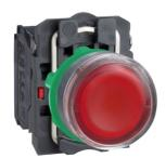
Illuminated push button, Harmony XB5, plastic, flush, red, 22mm, plain lens for BA9s bulb, spring return, lower than 250V, 1NO + 1NC
