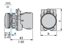
$\boldsymbol{e}\text{:}$  clamping thickness: 1 to 6 mm / 0.04 to 0.24 in.
