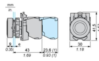
e: clamping thickness: 1 to 6 mm / 0.04 to 0.24 in. (1) Additional row of contacts or double contact
