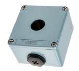
Harmony XAP, XB2 SL, Empty control station, zinc alloy, blue, 1 cut-out, Ø22, with ISO cable entries, 80 x 80 x 51.5 mm
