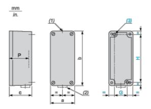
(1) 1 hole, without blanking plug, for cable gland with 18 mm/0.71 in. maximum clamping capacity
