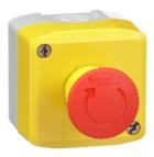
Control station, Harmony, plastic, yellow, 1 red mushroom head push button 40mm, emergency stop turn to release 2 NC, unmarked, UL CSA certified
