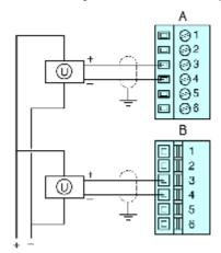
2 non-isolated analog sensors, 24 VDV supplied by the PDM  $\,$
