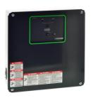
Surge protection device, Surgelogic, 320kA, 600 VAC delta, 3 phase, 3 wire, NEMA 1, disconnect switch
