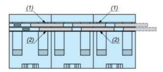
(1) 2 bus jumpers (polarity A2)(2) 2 bus jumpers (polarity A1)
