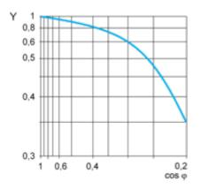
Y Reduction coefficient (A) Maximum switching capacity on resistive DC load
