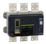
Circuit breaker, PowerPacT R, 1600A, 3 pole, 600VAC, 50kA, busbar, Micrologic 5.0P, 80%, modbus
