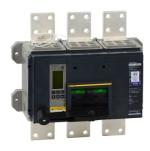
Circuit breaker, PowerPacT R, 1600A, 3 pole, 600VAC, 50kA, busbar, Micrologic 5.0P, 100%, modbus
