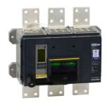
Circuit breaker, PowerPacT R, 600A, 3 pole, 600VAC, 50kA, busbar, Micrologic 5.0P, 80%, modbus
