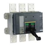
Circuit breaker, PowerPacT R, 2000A, 3 pole, 600VAC, 65kA, busbar, Micrologic 5.0, 100%
