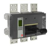
Circuit breaker, PowerPacT R, 600A, 3 pole, 600VAC, 65kA, busbar, Micrologic 5.0H, 100%, modbus
