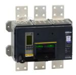
Circuit breaker, PowerPacT R, 1600A, 3 pole, 600VAC, 25kA, busbar, Micrologic 5.0P, 80%, modbus
