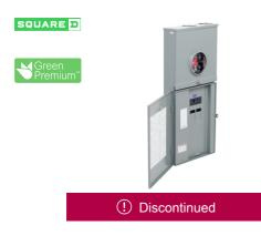
Meter mains, Homeline, CSED, ringless socket, 200A, surface mount, maximum 8 spaces, 16 circuits, horn bypass
