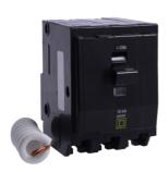
Mini circuit breaker, QO, 15A, 2 pole, 120VAC, 10kA, plug in, switch neutral, 50 deg C
