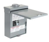
Generator panel, QO, 1 phase, 4 spaces, 8 circuits, 20A main breaker with interlock, NEMA3R, gnd bar, UL
