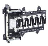
Load center interior, QO, 1 phase, 32 spaces, 32 circuits, 100A convertible main breaker, NEMA1, UL
