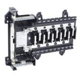
Load center interior, QO, 1 phase, 20 spaces, 24 circuits, 125A convertible main lugs, NEMA1, gnd bar, UL
