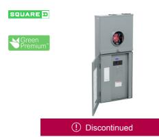
Meter mains, QO, CSED, ringless socket, 150A, outdoor surface mount, maximum 8 spaces, 16 circuits, lever bypass
