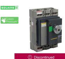
Automatic switch, PowerPacT P, 600A, 3 pole, 600VAC, 25kA, lugs, magnetic, black rotary handle
