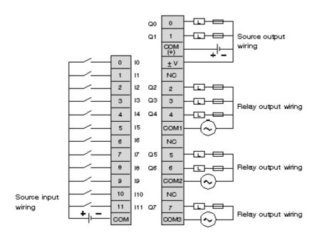
• Output points 0 and 1 are source transistor outputs, all other output points are relay.
