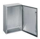
Wall mounted enclosure, Spacial S3X, stainless steel 316L, plain door, 300x300x150mm, IP66
