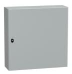
Wall mounted steel enclosure, Spacial S3D, plain door, with mounting plate, 800x800x250mm, IP66, IK10
