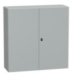
Wall mounted steel enclosure, Spacial S3D, double plain door, with mounting plate, 1200x1200x400mm, IP55, IK10
