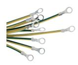
Earth leads section 10mm<sup>2</sup>, length 170mm, eyelet hole 8,3mm. Packaging unit: 10.
