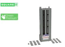
Panelboard interior, NQ, main lugs, 225A, Al bus, 72 pole spaces, 1 phase, 3 wire, 240VAC, 48VDC
