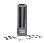
Panelboard interior, NF, main lugs, 250A, Cu bus, Al neutral assembly, 54 pole spaces, 3 phase, 4 wire, 600Y/347VAC max
