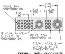
ENDWALL WITH KNOCKOUTS (OTHER ENDWALL IS BLANK)
