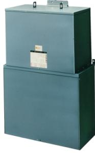
Unit substation, Mini Power-Zone, plug on, 15kVA, 3 phase, 480V primary, 208Y/120V secondary, 18kA, C, stainless steel
