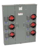
Meter center, MP Meter-Pak, 6 sockets, no bypass, 5 jaws, 600A bus, 125A max breaker rating, ringless
