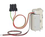
XF closing voltage release, MasterPact MTZ2/MTZ3 drawout, diagnostics and communicating, 48VAC 50/60Hz, 48/60VDC
