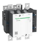
TeSys F contactor - 3P (3 NO) - AC-3 - <= 440 V 150 A - coil 380V AC
