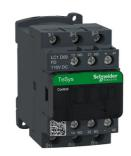
IEC contactor, TeSys Deca, nonreversing, 9A, 5HP at 480VAC, up to 100kA SCCR, 3 phase, 3 NO, 110VDC coil, open style
