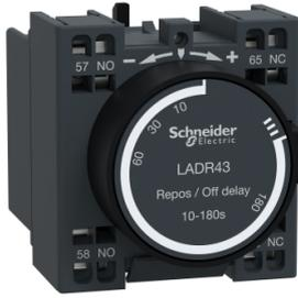
Time delay auxiliary contact block, TeSys Deca, 1NO + 1NC, off delay 10-180s, front, spring terminals
