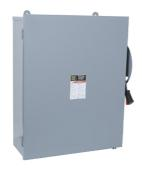
Safety switch, heavy duty, non fusible, 200A, 4 pole, 150HP, 600V AC/DC, NEMA 12
