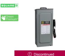
Safety switch, heavy duty, non fusible, 30A, 4 wire, 3 pole, 1 neutral, 30HP, 600V AC/DC, NEMA 3R, bolt on hub provision
