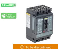
Circuit breaker, PowerPacT H, 110A, 3 pole, 600VAC, 50kA, lugs, thermal magnetic, 80%, interchangeable trip unit
