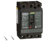
Circuit breaker, PowerPacT H, 20A, 3 pole, 600VAC, 50kA, lugs, thermal magnetic, 80%
