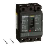
Circuit breaker, PowerPacT H, 70A, 3 pole, 600VAC, 18kA, lugs, thermal magnetic, 80%
