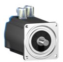
servo motor BSH, Lexium 05, 11.1N.m, 1500rpm, 140mm, untapped shaft, Sincos single turn, without brake, IP50
