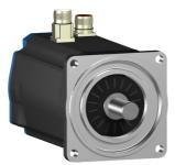
AC servo motor BSH, Lexium 05, 9.31N.m, 1500rpm, keyed shaft, with brake, IP65
