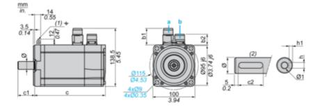
a: Power supply for servo motor brake
