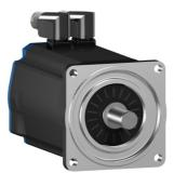
servo motor BSH, Lexium 05, 9.31N.m, 1500rpm, 100mm, untapped shaft, Sincos single turn, without brake, IP50
